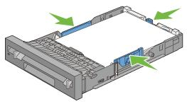
NOTE: When loading user-specified print media, adjust the width guides and slide the extendable part of the tray by pinching the length guide and sliding it until it rests lightly against the edge of the paper.
